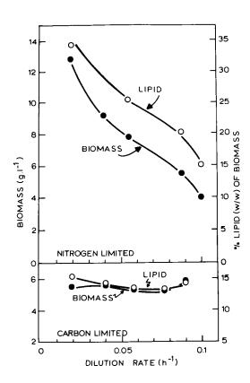
Fig. 1. Biomass production and lipid accumulation in  $R.\ glutinis$  growing in continuous culture. Nitrogen-limited medium contained (g litre<sup>-1</sup>) glucose 30, NH<sub>4</sub>Cl 1.5 and yeast extract (11% N content) 1.5; carbon-limited medium contained glucose 12, NH<sub>4</sub>Cl 3.0 and yeast extract 1.5.
