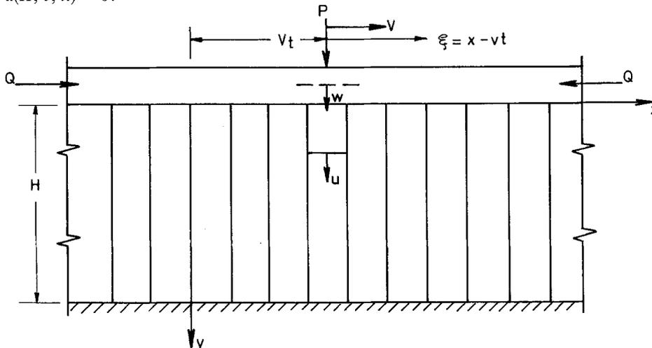
Fig. 1. Beam-foundation system
