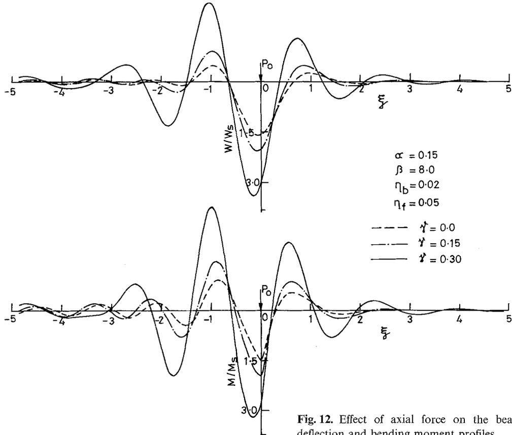
Fig. 12. Effect of axial force on the beam deflection and bending moment profiles
