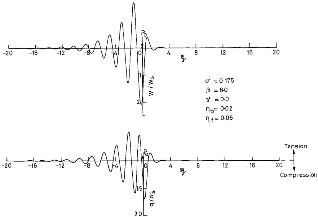
Fig. 16. Profiles of beam deflection and foundation pressure
