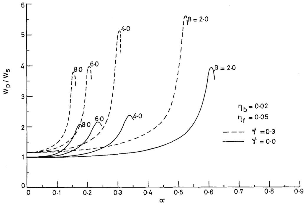
Fig. 8. Effect of velocity on peak beam deflection
