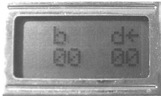
Fig. 3. The Hummingbird display. This device, a, has detected devices b and d. The arrow indicates that device d was the latest one to be detected. The numbers are an indication of signal strength, used for debugging purposes.
