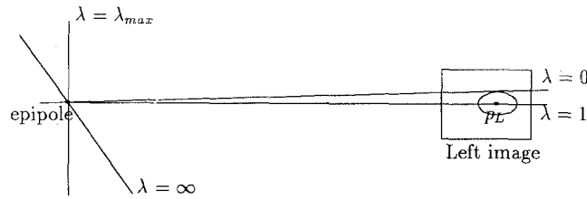
Fig. 4. The normal situation. The distance between the point p_L and the epipolar line for \lambda = 0 is much smaller than the distance to the epipolar line for \lambda = \infty and much smaller than the distance to the epipole. Note that the distances are measured using the covariance matrices. This implies that all points on the drawn ellipse lie at the same distance from the point p_L , which is the center of the ellipse.
