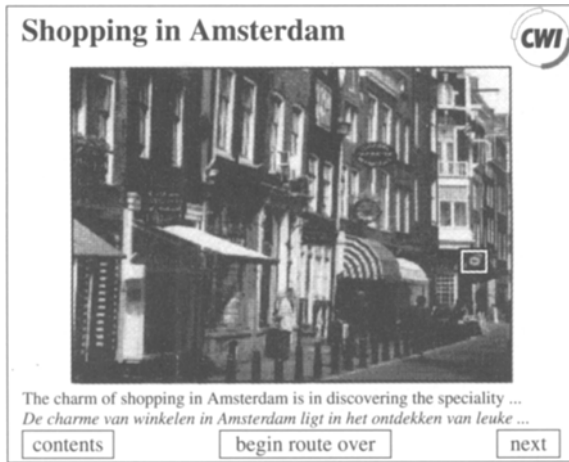
Fig. 2. An example multimedia application. The rectangles along the bottom represent navigation controls; the square in the picture is a hyperbutton. The two lines of text are captions that accompany multilingual audio
