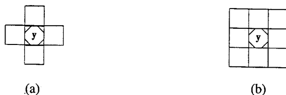
Figure 3. (a) The von Neumann or 4-neighborhood of y ; (b) the Moore or 8-neighborhood of y .
