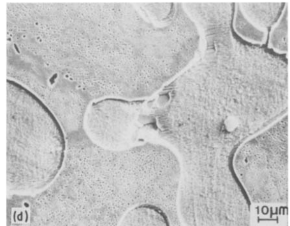
Figure 7 Microstructures of some slowly cooled doped (1 at.%) eutectic alloys ( 5^\circ\text{C min}^{-1} ). (a) Fe, (b) Al, (c) Ti, (d) V.
