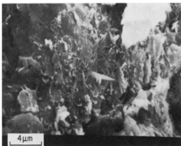
Figure 9 Scanning electron micrograph of the fracture surface of 12 week (75°C) cured soil-10 wt % lime sample, \times 3500 .
