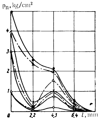
Fig. 3. Dependence of the distribution of the hydrodynamic pressure of AK-10 oil in the clearance between friction elements on the pressure of the liquid being sealed and on the specific pressure at v_{av} = 3 m/sec, l = 8.5 mm: \cdots p_s = 5 kg/cm 2 ; \text{---} p_s = 2 kg/cm 2 ; \circ p_n = 1 kg/cm 2 ; \Delta p_n = 3 kg/cm 2 ; \times p_n = 4 kg/cm 2 ; \bullet p_n = 5 kg/cm 2 .
