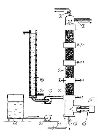
Fig. 1 : Device for continuous extractive fermentation coupling liquid-liquid extraction and ethanol production by immobilized cells.
