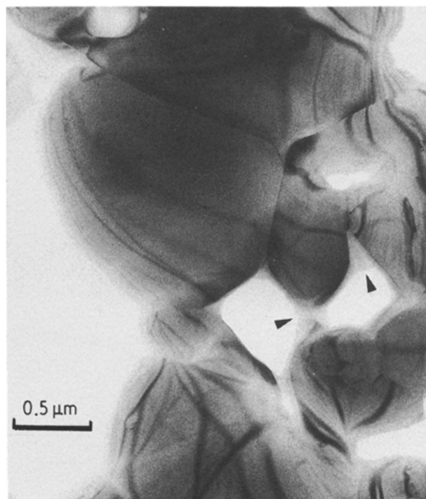
Figure 3 Microstructure of mullite grains from Af-Sc sample fired at 1550 °C for 44 h. Arrows point towards unreacted silica around pores. Notice the absence of intergranular silica.
