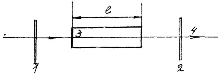
Fig. 5. Nonlinear filter based on self-induced rotation of the polarization plane: 1, 2) polarizers crossed at an angle  $\varphi_0$ ; 3) "rotating" sample; 4) light beam.
