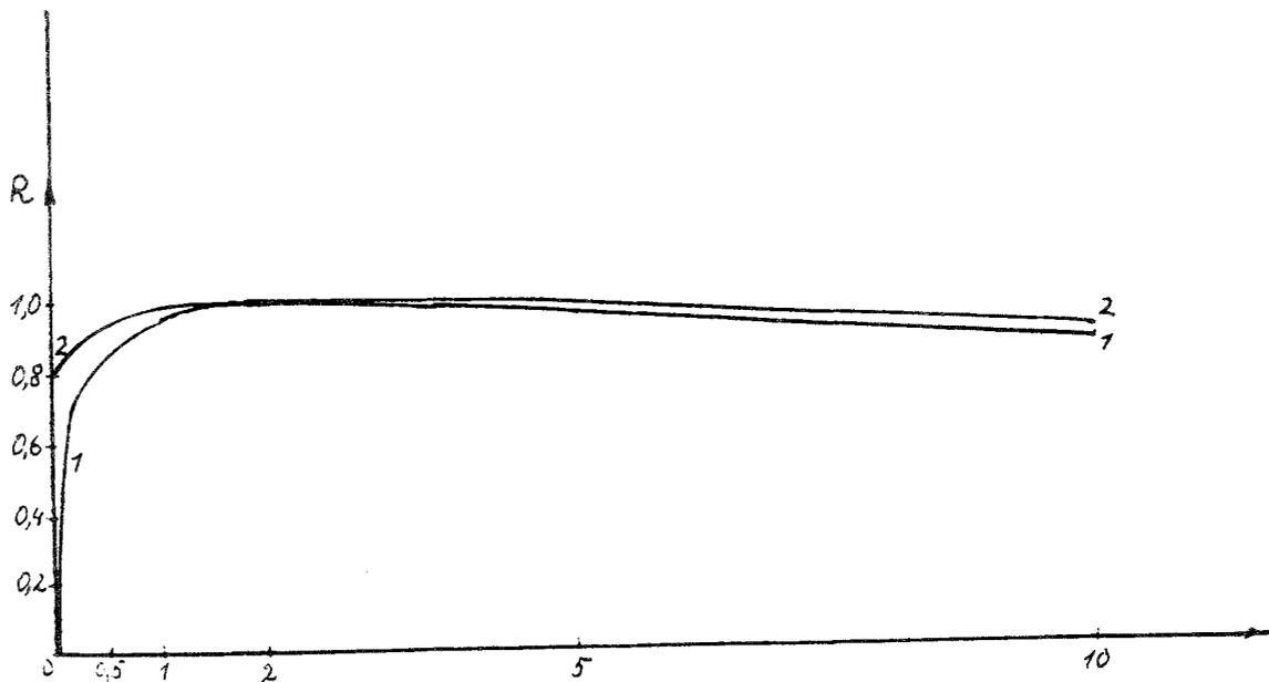
Fig. 4. Transmission in refraction close to the TIR angle on the interface of a linear and nonlinear medium;  $n_{10} = 1.3003$ ,  $n_{20} = 1.30000$ ,  $\kappa = 2 \cdot 10^{-11}$ ; TIR angle  $\varphi_0 = 88.77^\circ$ ; curve 1 corresponds to  $\Delta = 0$  and curve 2 to  $\Delta = 0.1^\circ$ .
