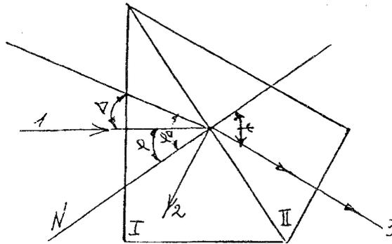
Fig. 3. Refraction, in a prism, near the total internal reflection angle. 1) prism of linear material; 2) prism of nonlinear material; 3) normal to the interface of the media;  $n_{10} \geq n_{20}$ ;  $\varphi_0$ ) total internal reflection angle ( $\sin \varphi_0 = n_{20}/n_{10}$ );  $\varphi$ ) incidence angle;  $\psi$ ) refraction angle; 1, 2, 3) incident, reflected, and refracted beams, respectively.
