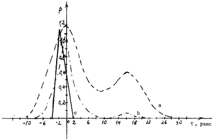
Fig. 10. Mode locking under conditions of "hard" start: a) dashed, initial profile, for left-hand spike  $\tau = 10$  psec,  $p_0 = 0.12$ , M1:0.1; b) dashed, 5th pass,  $\tau = 5$  psec, M1:3; c) solid, 8th pass,  $\tau = 2.5$  psec, M1:600
