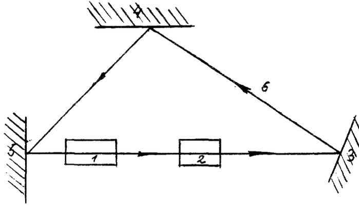
Fig. 8. Diagram of traveling-wave laser in a ring cavity with nonlinear element: 1) active element; 2) nonlinear element; 3, 4, 5) mirrors; 6) light beam.
