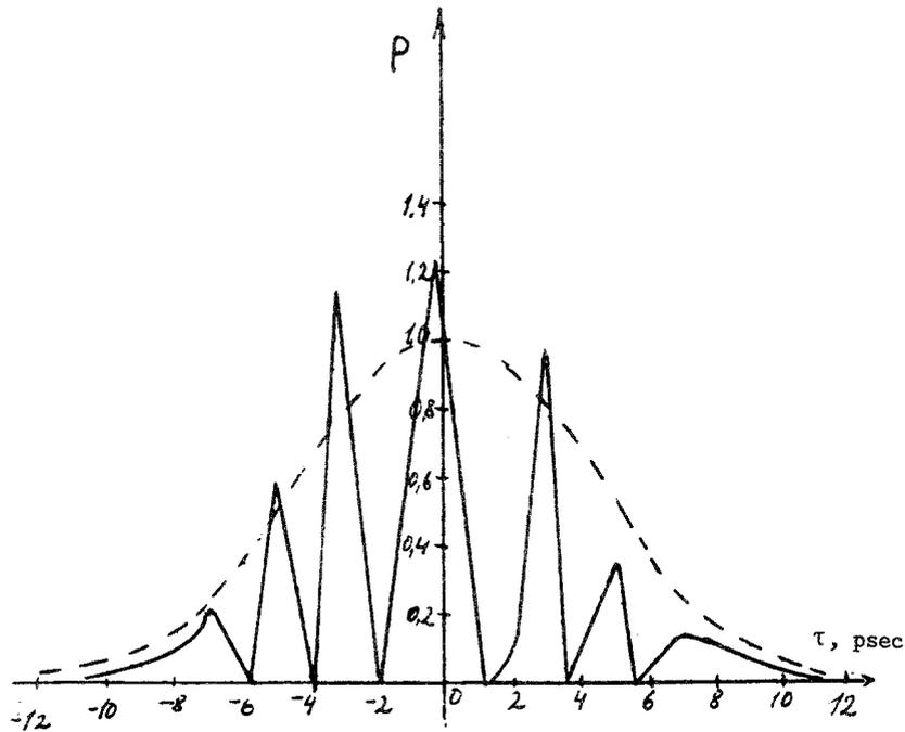
Fig. 12. Breakup of pulse by a nonlinear element based on SIRPP; a) initial pulse, M1:1; b) pulse in second pass, M1:50.
