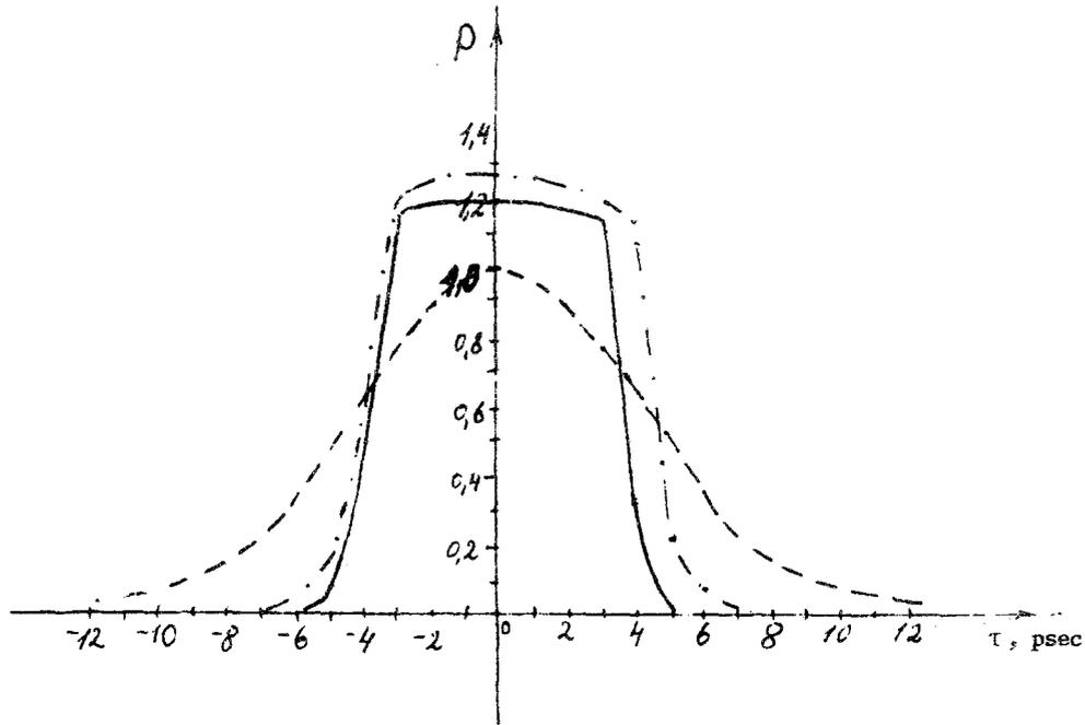
Fig. 11. Generation of square pulses with the aid of an element with self-induced rotation of the polarization plane: a) initial pulse; b) pulse in 4th pass; d) pulse in 6th pass.
