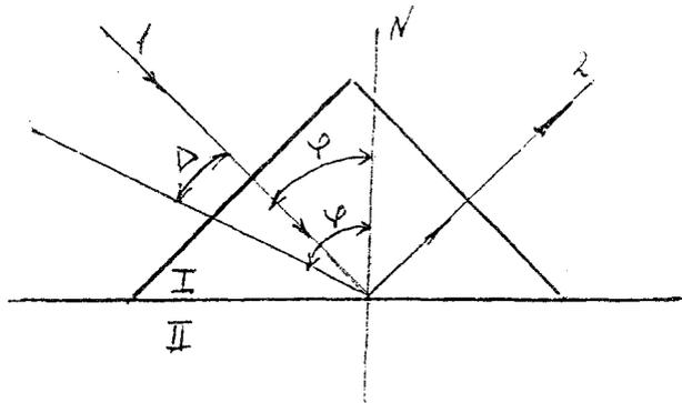
Fig. 2. Reflection under conditions close to TIR. I) prism of nonlinear material; II) medium of linear material ( $n_{20} < n_{10}$ ),  $\varphi_0$ ) total internal reflection angle ( $\sin \varphi_0 = n_{20}/n_{10}$ );  $\varphi$ ) incidence angle,  $\varphi = \varphi_0 - \Delta$ ; N — normal; 1, 2) incident and reflected rays.
