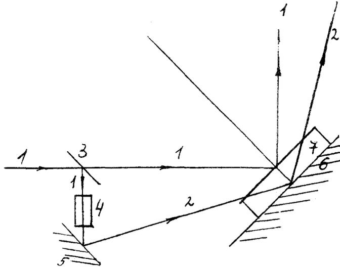
Fig. 6. Nonlinear element based on self-rotation of polarization ellipse: 1, 5) polarizers crossed at an angle  $90^\circ$ ; 2, 4) crystalline phase plates; 3) "rotating" sample; 6) beam.
