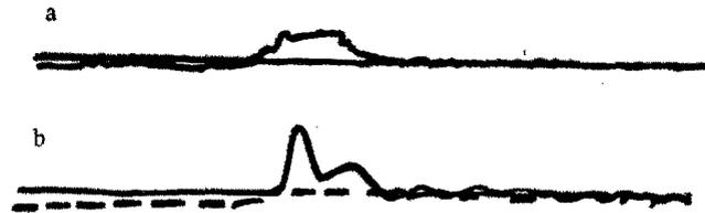
Fig. 12. Oscilloscope of 20-nsec pulse past the driver laser (a) and at the exit from one of the power amplifier channels (b).
