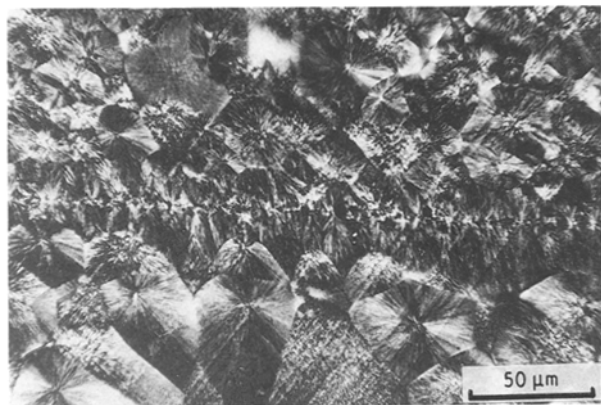
Figure 8 Later-particle microstructure of sintered Propathene GSE 16 polypropylene.
