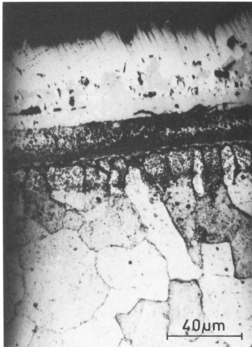
Fig. 7. Optical micrograph showing the formation of internal oxides both within and on the grain boundaries (Nital etch) on a 37% cold-worked sample oxidized for 4 hr at 900°C.
