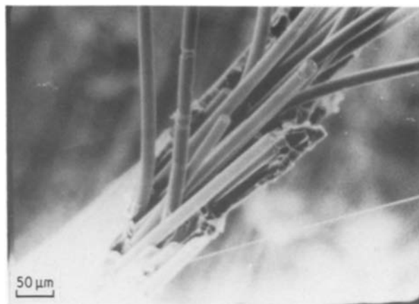
Figure 13 Fracture morphology of filament-PEEK composite.
