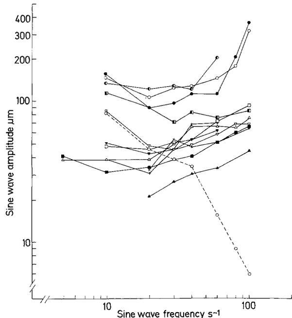
Fig. 3. Tuning curves for 12 rapidly adapting mechanoreceptors from the superficial branch of the left radial nerve in human subjects (solid lines) and the human threshold function for the perception of sine wave oscillation applied to the hairy skin of the hand (dashed line). A point in the latter curve represents the mean of 10 subjects. 5 determinations of thresholds were made in each subject
