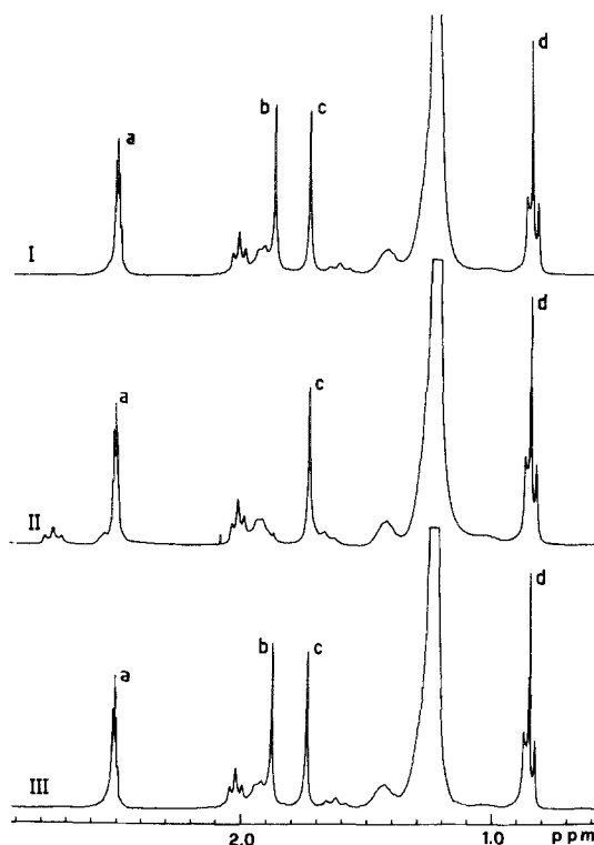
Figure 1. 300 MHz proton NMR spectra of the starting material, natural GM1 (I); GM1 after de- N -acetylation (compound 1) (II); reconstituted GM1 (compound 1 after re- N -acetylation) (III). Peak a, dimethylsulphoxide; peak b, acetyl protons of N -acetylneuraminic acid; peak c, acetyl protons of N -acetylgalactosamine; peak d, methyl protons of the alkyl region.
