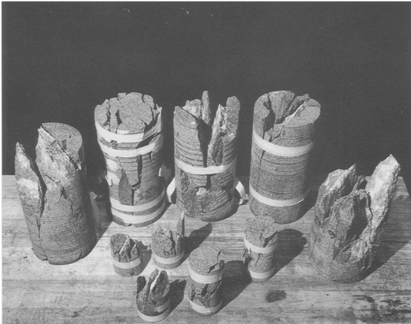
Fig. 1. UC tests-fractured specimens 70 and 145 mm diam.
