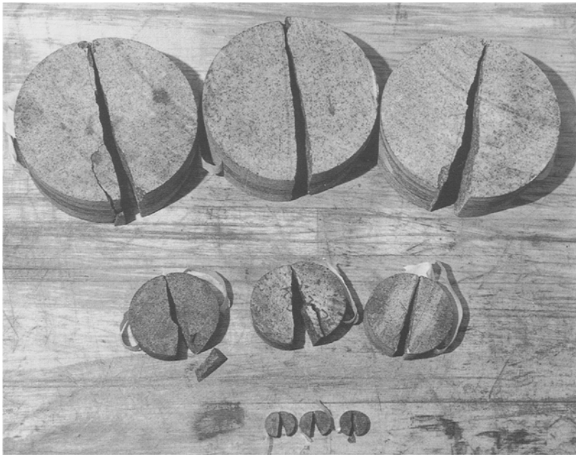
Fig. 3. DC tests-fractured specimens 21, 70 and 145 mm diam.
