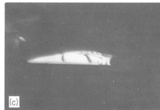
Figure 1 A grain boundary region in AISI 310, 50% deformed and annealed for 60 sec at 1173 K: (a) small twinned volume at the boundary, with the coherent twin interface arrowed and an M_{23}C_6 precipitate visible at A, (b) 200 matrix dark-field image of the region shown in (a) and (c) 1\ \bar{1}\ 1 twin dark-field image of the region shown in (a).
