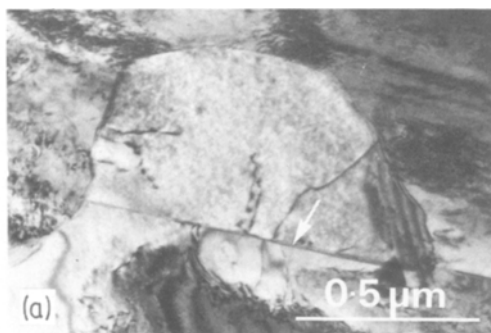
Figure 2 A \Sigma 3 twin oriented bulge on a grain boundary in 50% rolled \alpha -brass annealed for 1800 sec at 573 K: (a) the coherent twin interface is arrowed, (b) the same area as in (a), but tilted to show more clearly the discontinuity in dislocation density across the coherent twin interface (arrowed) and (c) \langle 110 \rangle axis selected area diffraction patterns from the boundary region shown in (a) and (b). In this pattern the common \langle 1\bar{1}1 \rangle for the twin and parent grains is indicated along A while the nearly common \langle \bar{1}11 \rangle of the twin and the grain into which the bulge is growing is indicated along B.
