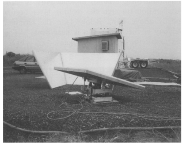
Fig. 3. The 915 MHz wind profiler and Integrated Sounding System (ISS) constructed for the Tropical Ocean Global Atmosphere (TOGA) Program and used in support of the Coupled Ocean Atmosphere Response Experiment (COARE). The electronically-steered phased-array antenna is mounted in the roof of a modified shipping container and is surrounded by a clutter screen
