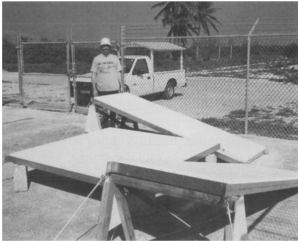
Fig. 1. The original 915 MHz wind profiler installed at Christmas Island in early 1990. Shown are the three microstrip antennas fixed to look in different directions
