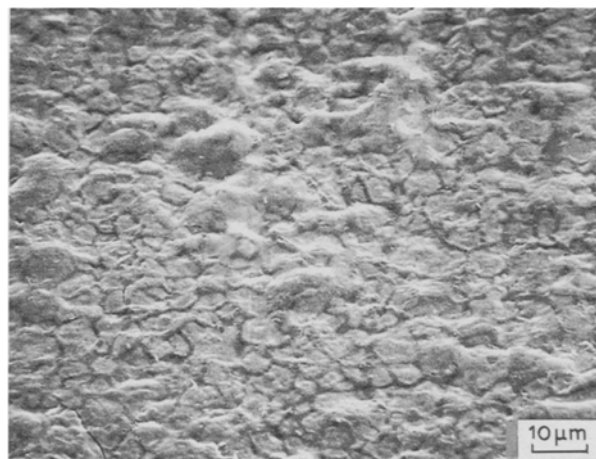
Fig. 1. SEM surface micrograph of a polyaniline film obtained on mild steel. Basic solution \text{H}_2\text{O}/\text{CH}_3\text{OH} : 50/50 vol %, \text{KOH} : 0.035 M; aniline: 0.3 M. Temperature 20°C no agitation. Potentiostatic: 1200 mV/SCE with 0.5 to 0.2 \text{A dm}^{-2} . Magnification \times 1000 .
