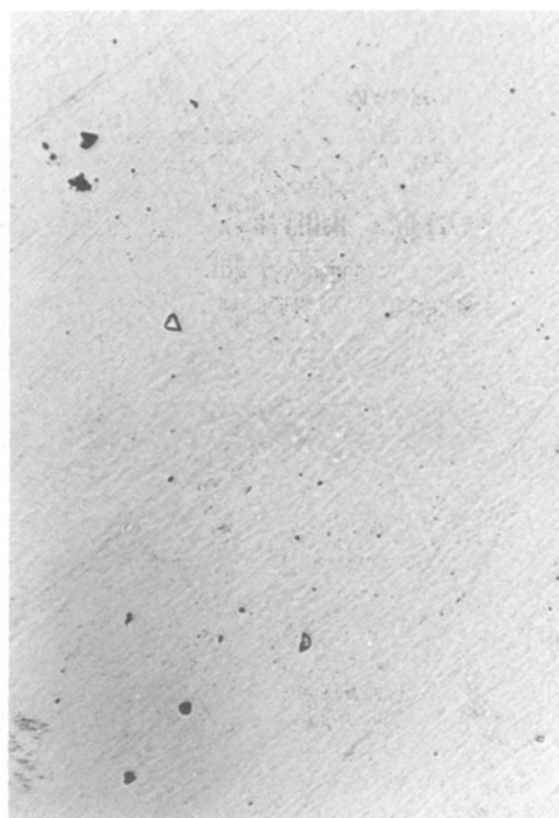
Figure 5 Optical micrograph of the single phase zone of the ingot (Alloy B).
