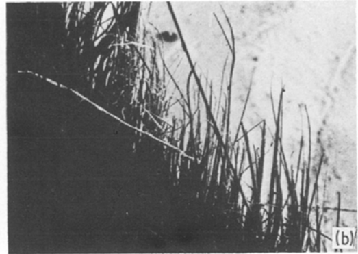
Figure 6 Pull-out in (a) glass, (b) Kevlar, and (c) carbon-fibre reinforced plastic.
