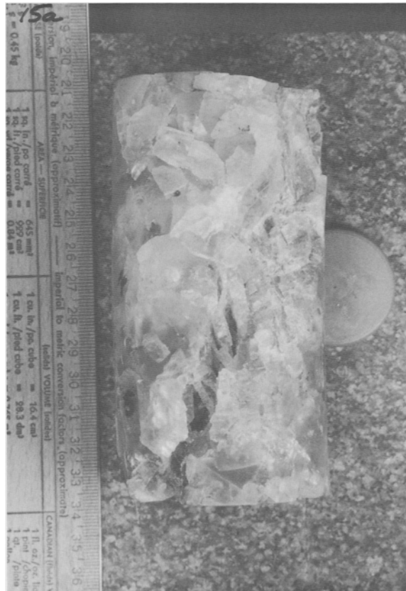
Fig. 9. The early stages of forming an inclined fracture is shown in this coarser grained, 120 mm high potash specimen coming from the Rocanville mine. Small slabs of rock are bounded by cleavage and form an en echelon shear crack-array. The rock slabs are in the early stages of buckling. Note the steep slope of the fracture array, only 25 degrees with the uniaxial loading direction
