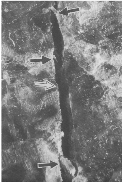
Fig. 8. A 30 mm long axial fracture in a cylindrical Lanigan potash specimen tested in triaxial compression. Note that the present fracture must have evolved through the union of several shorter segments (daughter cracks or step-outs), slightly offset from each other. The three black arrows point to rock bridges that are disintegrating. The white arrow marks a position where only a small jog suggests the position of an earlier step-out
