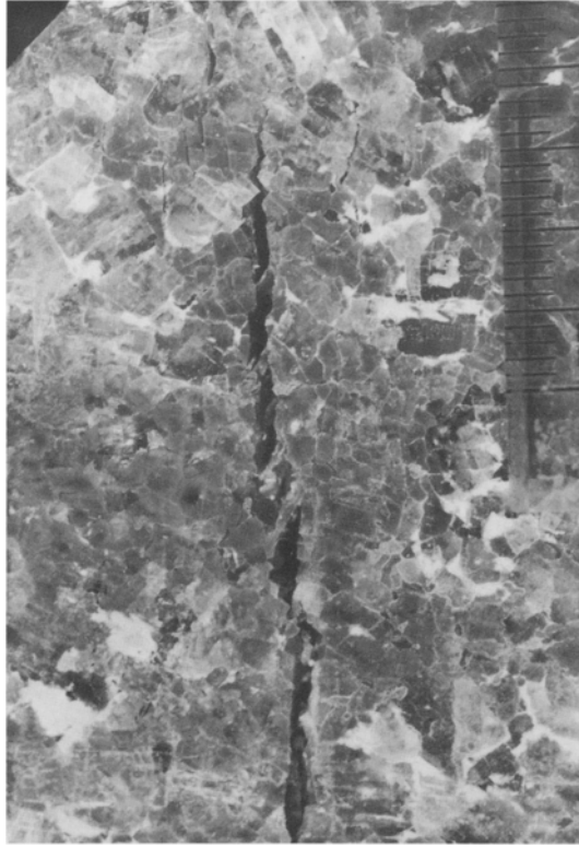
Fig. 13. Here the union of the members of an 80 mm en echelon tensile crack-array is almost complete. The site of the earlier step-out positions is however marked by the small rotated rock bridges
