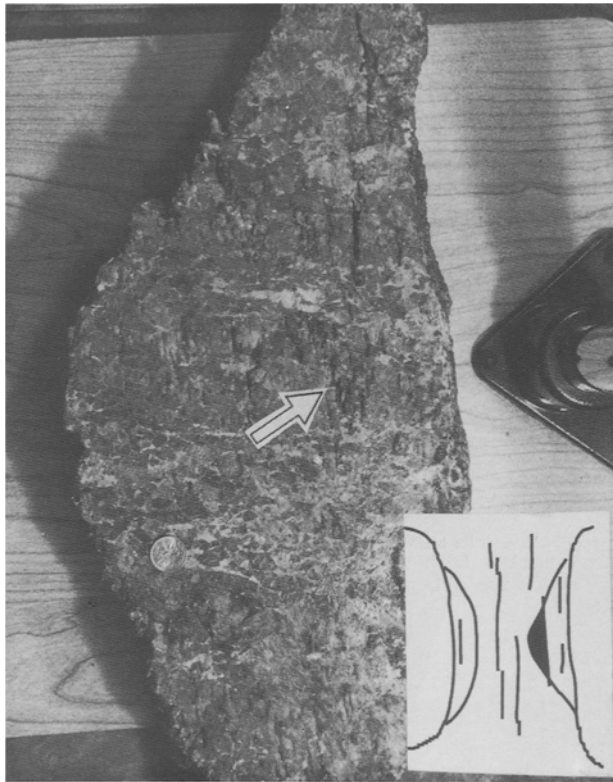
Fig. 4. Section of a 500 mm high block of rock removed from a failed pillar at the Central Canada Potash mine in Colonsay, Saskatchewan. On the left, the block is bound by an hourglass fracture; on the right, by a vertical tensile fracture. There are numerous, small tensile fractures inside the block and a few inclined structures that seem to parallel one or the other bounding surface on the left. The arrow points to an internal inclined en echelon shear crack-array. The sketch at the lower right corner shows the relative position of the block in the pillar
