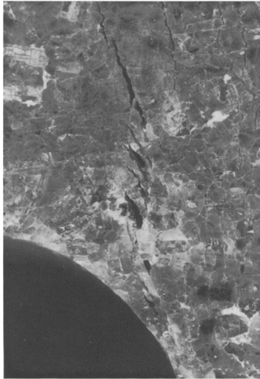
Fig. 14. Close to the perimeter of the cavity, the tensile cracks are shorter and the step-out is biased in one direction, away from the free surface. There is also a larger overlap between neighbouring cracks. As a result, a 30 mm long fracture zone formed, trending at an angle to the local principal stress direction
