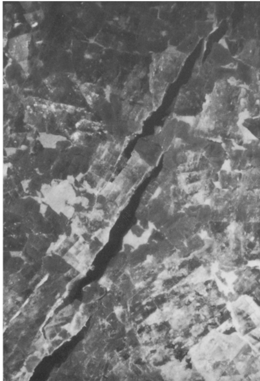
Fig. 12. A remote, en echelon tensile crack-array at two times magnification. The rock bridges are still well preserved, although buckling already commenced at the bottom
