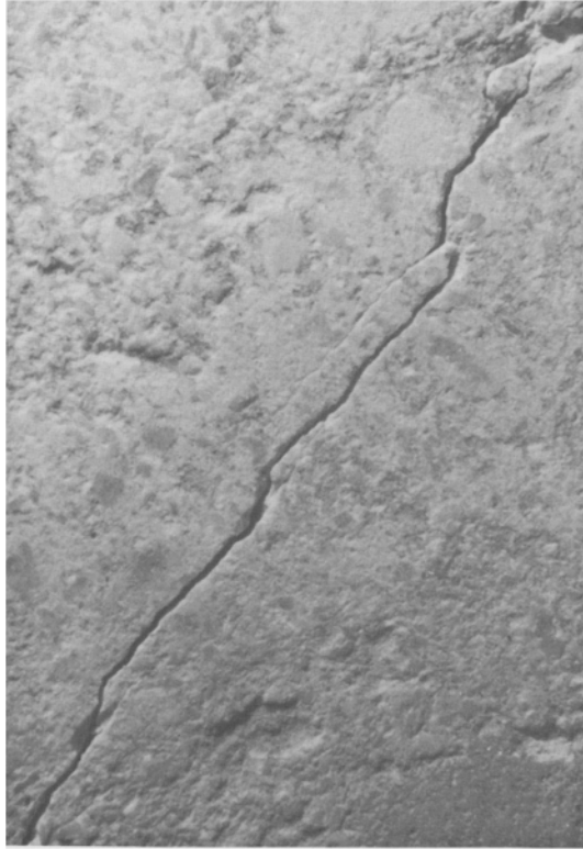
Fig. 20. A 70 mm long en echelon tensile crack-array in Tyndallstone, a relatively weak limestone. The (remote) fracture was produced in the laboratory while testing a limestone block with a central cavity. Here the rock bridges are destroyed by shearing through them
