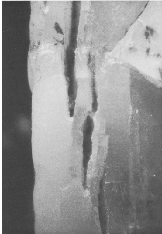
Fig. 18. An en echelon tensile crack-array in a single crystal of halite from the Central Canada Potash mine. The 100 mm wide single crystal has one of its cleavage planes oriented vertically. The three members of the en echelon tensile crack-array follow this cleavage direction. Courtesy of Dr. Alan Coode, Colonsay, Saskatchewan
