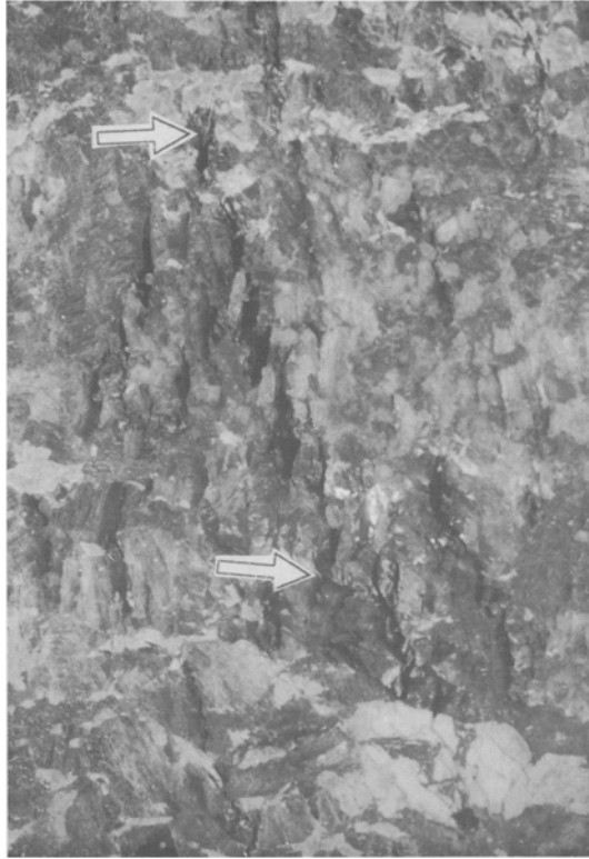
Fig. 21. An enlargement of the en echelon shear crack-array inside the potash block shown in Fig. 3. The arrows mark the two ends of the 100 mm long en echelon shear crack-array
