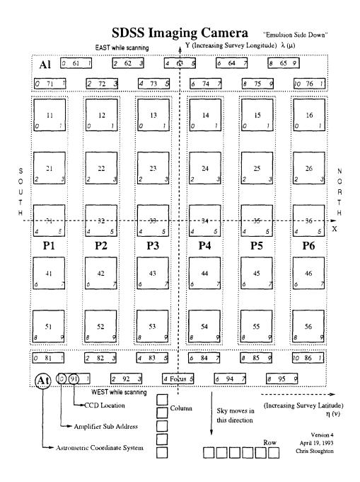
Fig. 1. Layout of the imaging camera focal plane.
