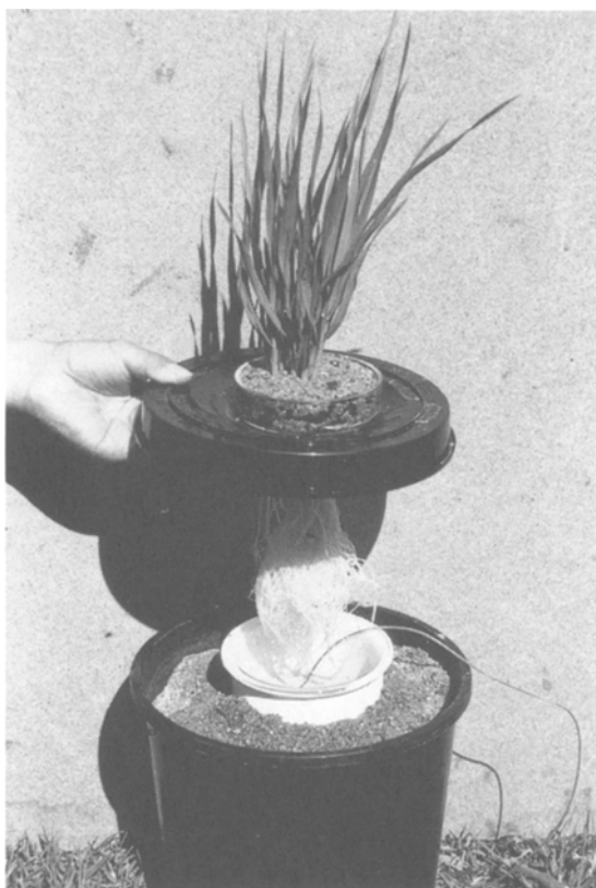
FIG. 2. Hydroponic system developed to study the release of allelochemicals by intact plants over time. The tube was connected to a RENA 301 air pump, which is not shown in the picture.
