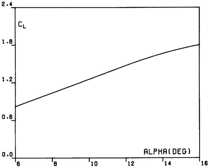
Fig. 1C. Lift coefficient  $C_L$  versus angle of attack  $\alpha$  for the Boeing B-727 aircraft (gear up, flap setting  $\delta_F = 15$  deg).
