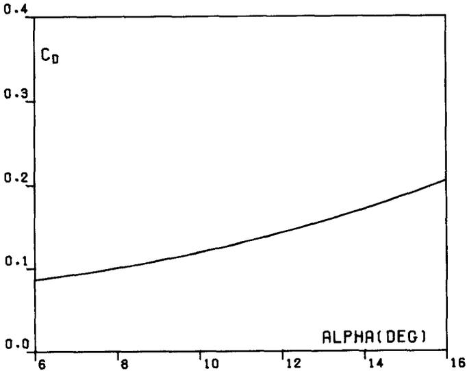
Fig. 1B. Drag coefficient  $C_D$  versus angle of attack  $\alpha$  for the Boeing B-727 aircraft (gear up, flap setting  $\delta_F = 15$  deg).
