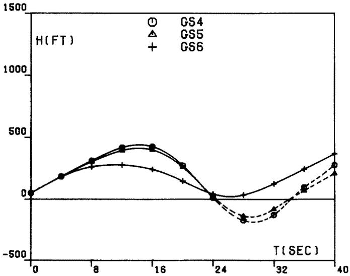
Fig. 4A. Particular guidance schemes: altitude  $h$  versus time  $t$ .
