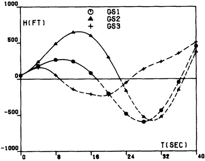
Fig. 3A. Particular guidance schemes: altitude  $h$  versus time  $t$ .
