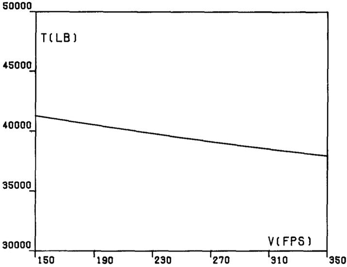
Fig. 1A. Thrust  $T$  versus velocity  $V$  for the Boeing B-727 aircraft powered by three JT8D-17 turbofan engines (maximum power setting, sea-level altitude, ambient temperature = 100 deg Fahrenheit).
