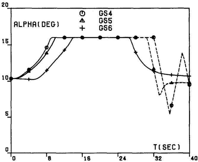
Fig. 4C. Particular guidance schemes: angle of attack  $\alpha$  versus time  $t$ .
