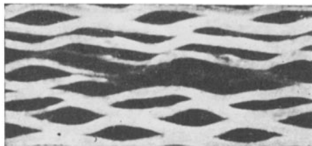
Fig. 5. Change in the distortion of the warp fibers when both warp and fill fibers are prestressed. Magnification 10\times . N_x = 0.1 R_M ; N_y = 0.1 R_M .
