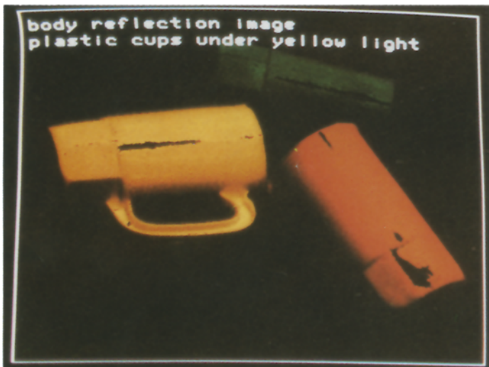
Color Figure 10. Intrinsic body reflection image of the three plastic cups under yellow light; clipped pixels and bloomed pixels are shown in black.
