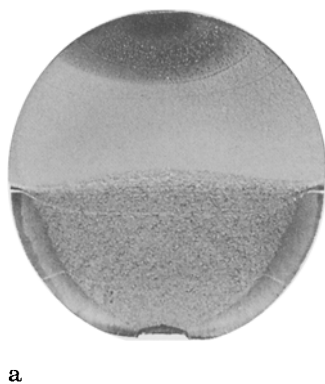
Fig. 5 and 6. 5a Photograph of the fractured cross-section of the V22-rotor. b Beach marks, drawn from the photograph of the cracked area; 6 Definition of the angle \alpha
