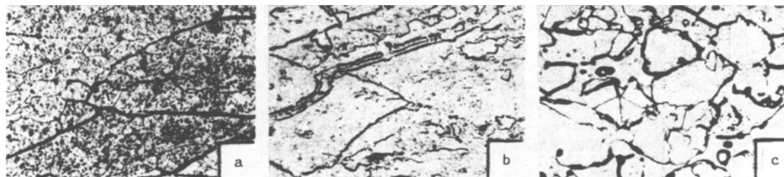
Fig. 1. Microstructure of corrosion-resistant steels after deformation at 1100^{\circ}\text{C} at rate \dot{\epsilon} = 8.3 \cdot 10^{-4} \text{ sec}^{-1} : a) 15Kh25T, \epsilon = 50\% , \times 100 ; b) 12Kh18N9, \epsilon = 75\% , \times 150 ; c) ÉK-72, \epsilon = 75\% , \times 250 .
