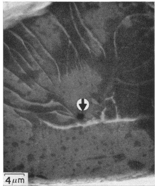
Figure 8 Showing at arrow a crack nucleation site. Note veins radiating from site.
