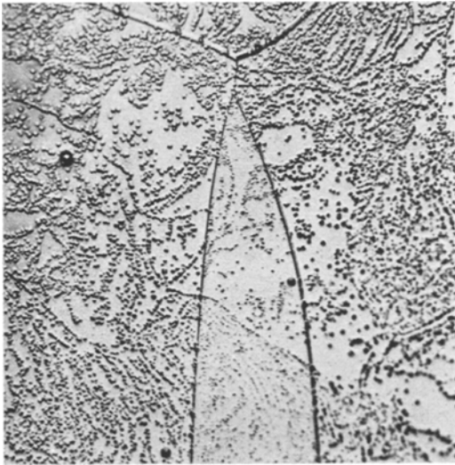
Figure 4 Polygonized dislocations in Armco iron deoxidized (AD) strained 3%, after anneal at 650°C (x660).
