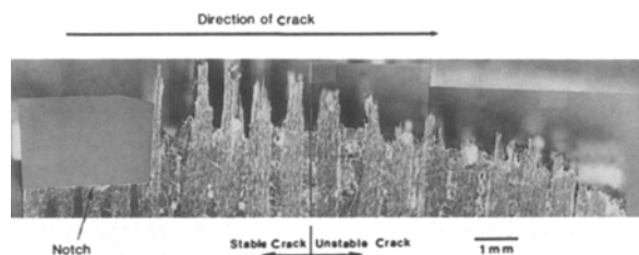
Figure 6 Photomicrograph of the bottom half of the fractured specimen of Fig. 5.
