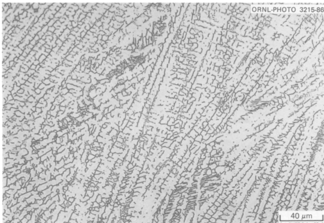
Fig. 1. Typical as welded microstructure of type 308 stainless steel.
