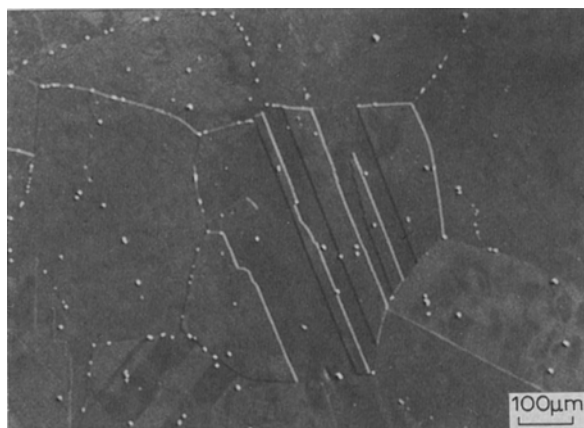
Figure 3 Lack of precipitation at twin boundaries.
