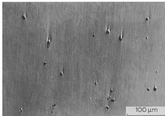
Figure 1 Ti-rich precipitates in as-received samples.
