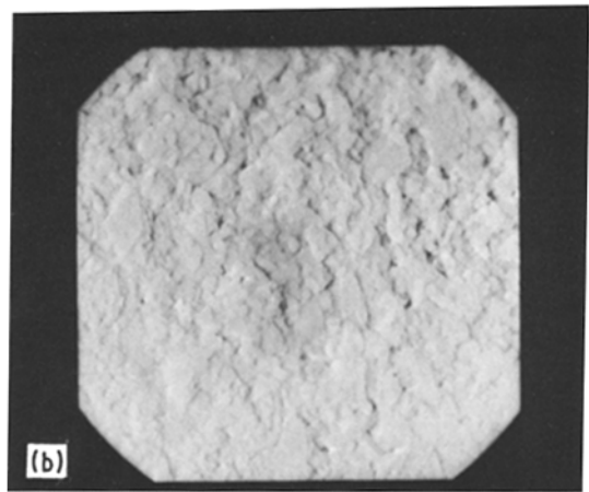
Figure 6 SEM of \text{Al}_2\text{O}_3 particles with (a) and without (b) \text{AlF}_3 at 1200^\circ\text{C} and 1 h ( \times 10000 ).
