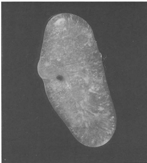
Figure 1 A solid piece of opaline silica (length 1 cm), showing diffraction colours, prepared by “drying” of silica suspension in silicone oil.
