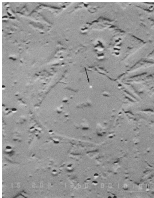
Figure 1 SEM micrograph of 2\text{CaO}\cdot\text{Si}_3\text{N}_4 phase which was analysed by electron probe (arrow point) with 45.6 wt % CaO:54.4 wt % \text{Si}_3\text{N}_4 \approx 2\text{CaO}\cdot\text{Si}_3\text{N}_4 ( \times 2000 ).
