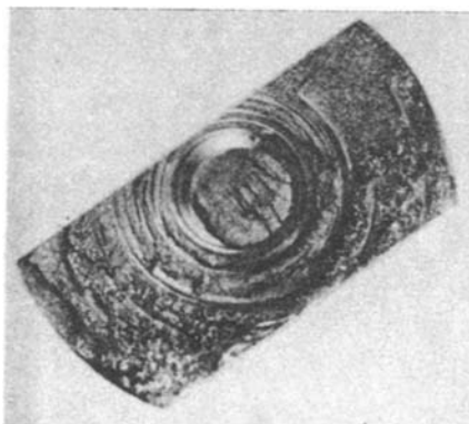
Fig. 1. "Bright rings" in the fracture of a tool blank.
