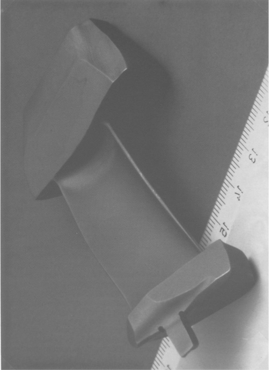
Figure 11. Gas turbine blade (blank piece). Material: PM 3030.
