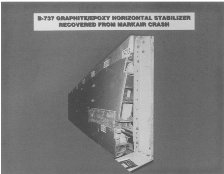
Figure 16. B-737 graphite/epoxy horizontal stabilizer recovered from Markair crash.
