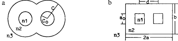
Fig. 2. (a) Cross-section of coupler made from fiber with disturbed cladding. (b) Rectangular model a_0 = \sqrt{\pi}C_0 , d = 2a - b
