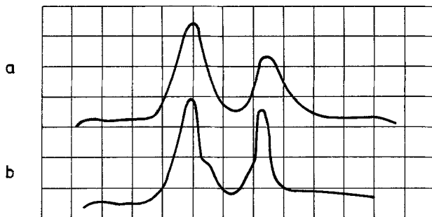
Fig. 6a and b. Oscilloscope traces of pump and signal 818 nm pulses. (a) Reference trace with pump pulse on input and output, (b) pump pulse on input and signal on output
