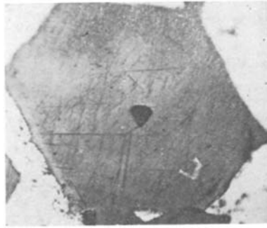
Fig. 2. Microstructure of Al + 20% Si with 0.6% P ( \times 1000 ).
