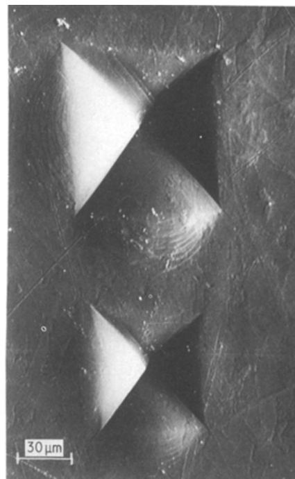
Figure 14 A normal incidence SEM view of two microhardness indentations produced in polystyrene under loads P of 83.3 and 166.6 g respectively.
