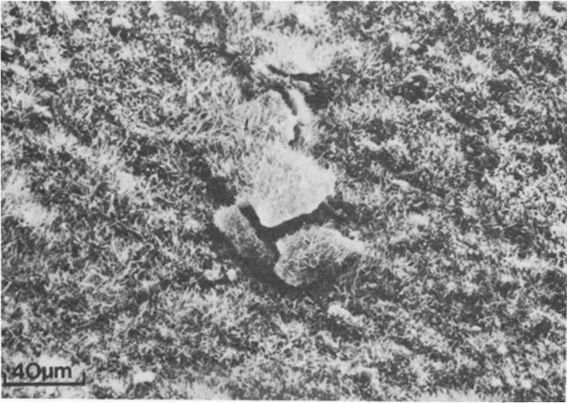
Fig. 5. RJM2012 outer scale after oxidation for 20 hr at 900°C.
