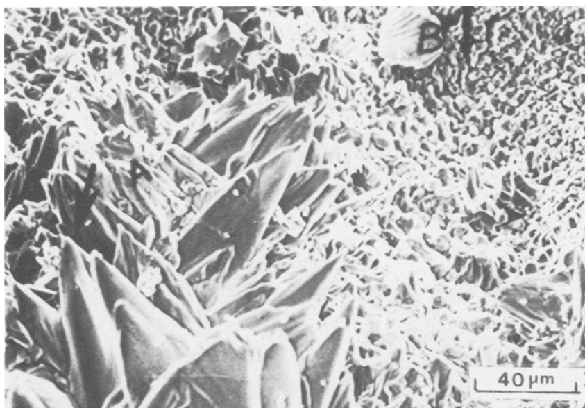
Fig. 19. Scale-gas interface for an Fe-25Cr alloy oxidized for 25 hr at 1150°C in air.
