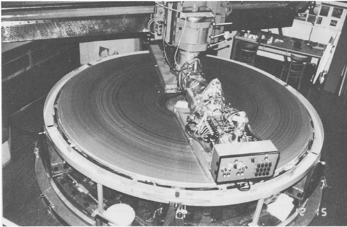
Fig. 4. Lapping the ESO-NTT primary with two rectangular tools.
